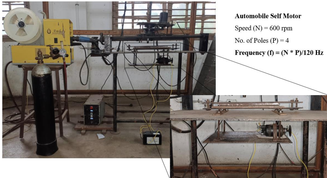
Figure 2 Rotational Arc Welding Apparatus with Vibrational Setup
