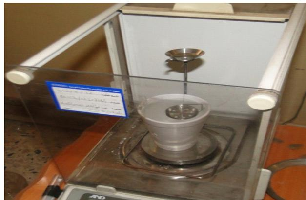
Fig. 2. mesh on the balance for measuring the weight hanging .
