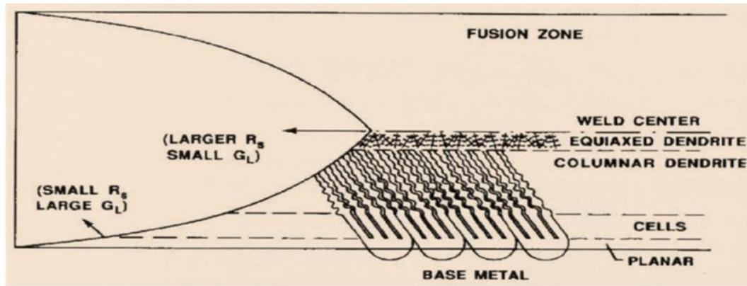
**Figure 3: Visual figure illustrating changes in configuration throughout the fusion zone across welding-type processes. ( $R_s$ =grain growth rate,  $G_L$  =thermal gradient in the liquid)**
