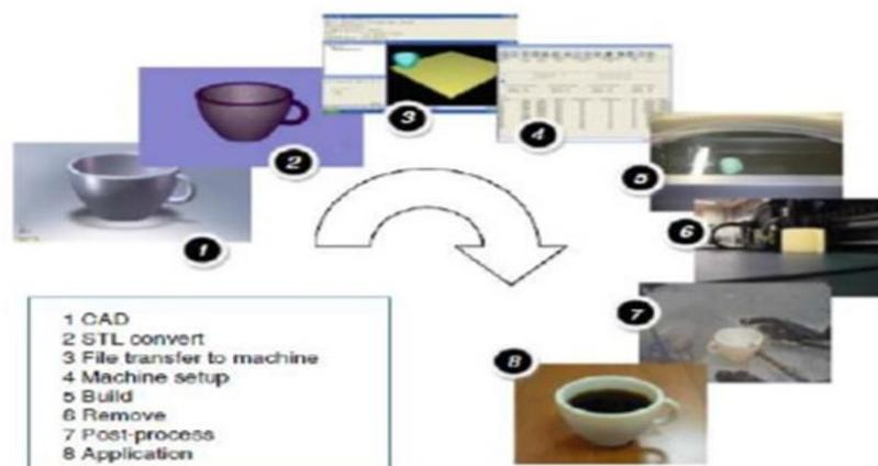
**Figure 1: The eight stages of the AM process [7]**
