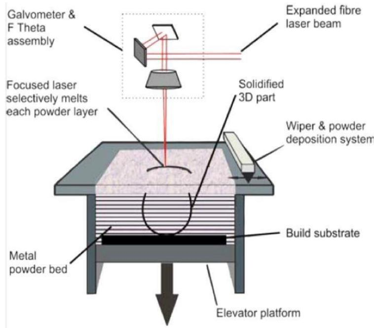
**Figure 4: Representation illustration of archetypal powder bed SLM system [57-58].**
