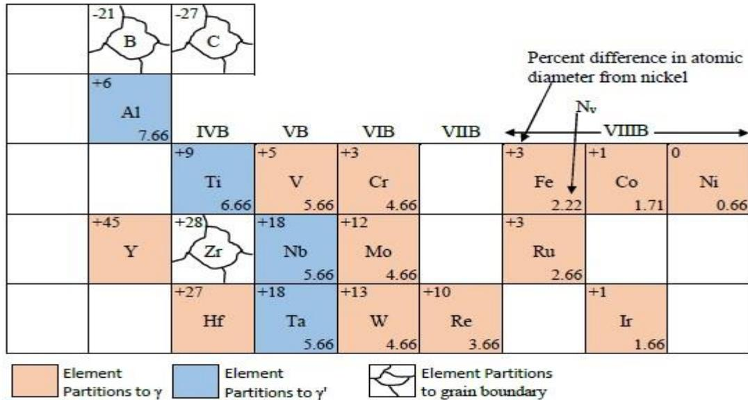
**Figure 2: Part of the periodic table of elements displaying metals used in superalloys and their clustering properties [49]**
