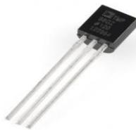
**Fig 1.1 TMP36 Temperature sensor**
