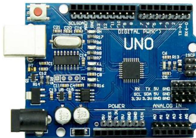
**Fig 1.4 Arduino R3 CH340G ATmega328p**
