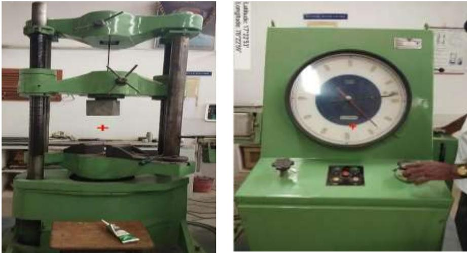
Fig 4. Experimental setup for finding the bond strength of the critical fiber content in triple blended SCC cube.
