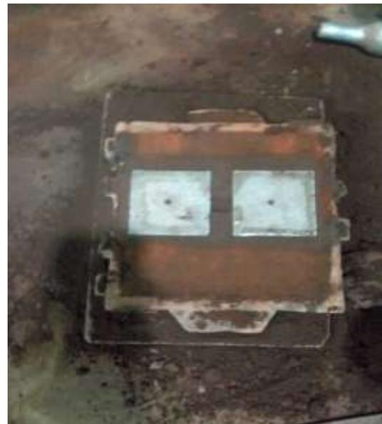
Fig. Pattern making in sand casting
