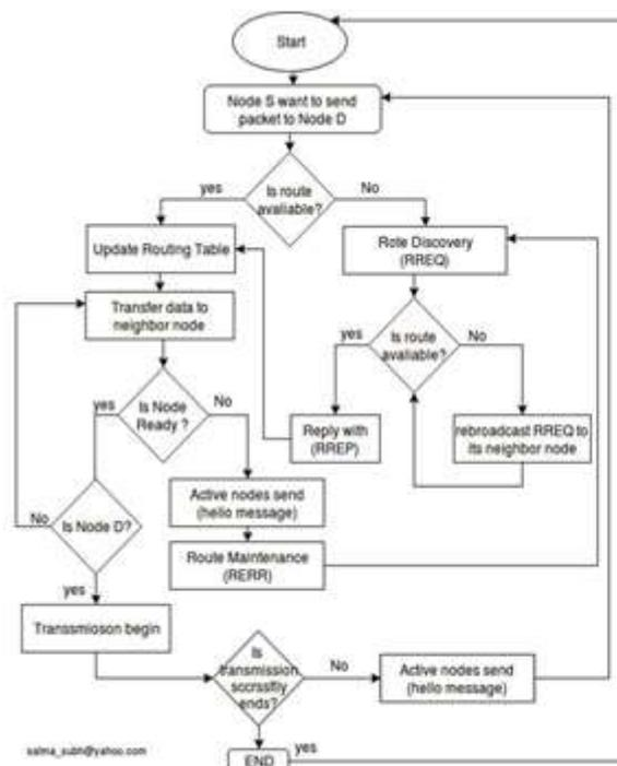
Figure 1. AODV algorithm flow chart
