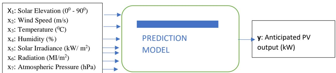
Figure 1. Solar PV Power prediction model
