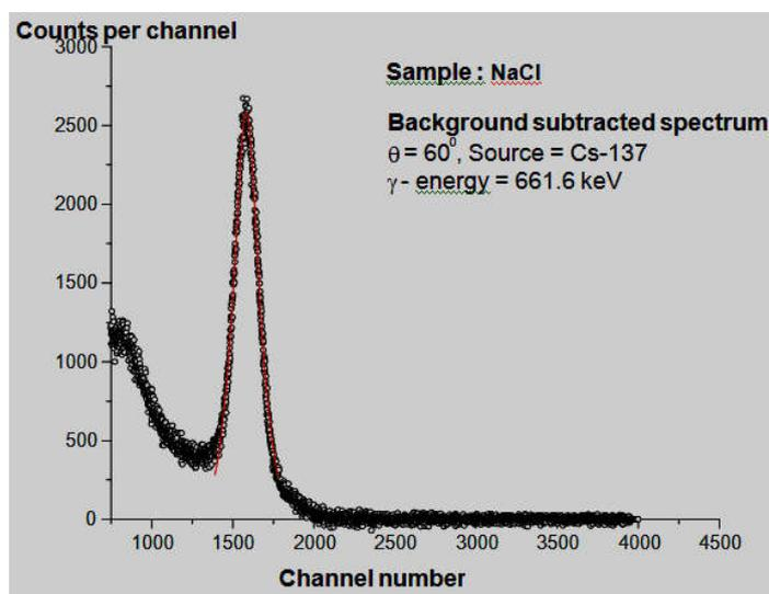
**Figure2: Back ground subtracted spectrum for NaCl at  $60^\circ$  and at 661.6keV**
