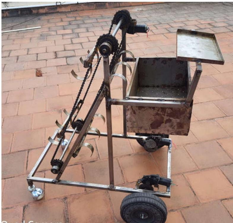
Fig.5.2 Side View Automatic Drainage Cleaning Machine
