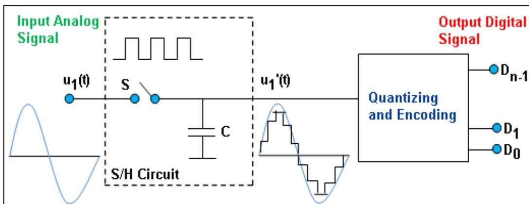
Figure 5. Complete AD Conversion Process
