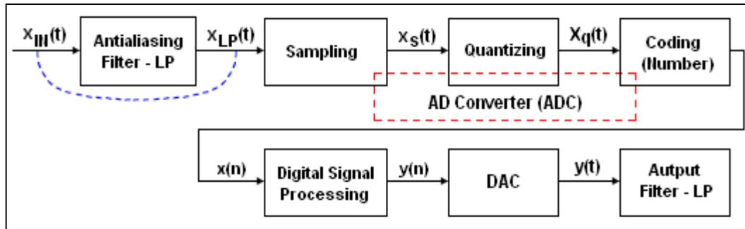
Figure 1. Block Diagram of Digital Signal Processing
