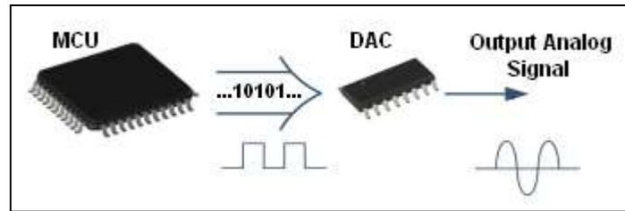
Figure 7. Cascade of the Circuit for DA Conversion
