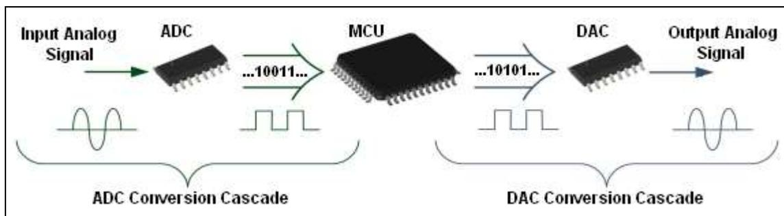
Figure 3. Solutions of AD and DA Processing Sequence
