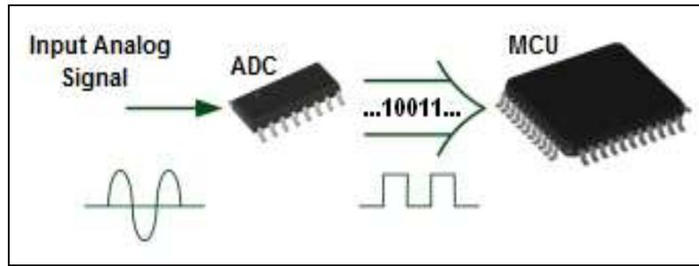
Figure 4. Cascade of the Circuit for AD Conversion
