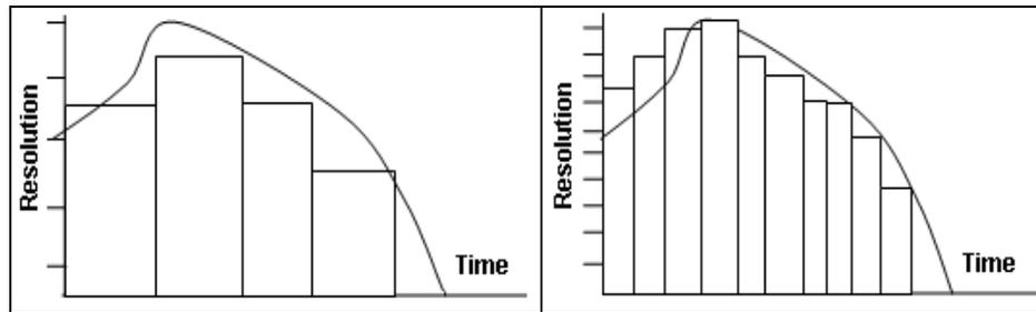
Figure 6. Low and Increased Accuracy of AD Conversion Process
