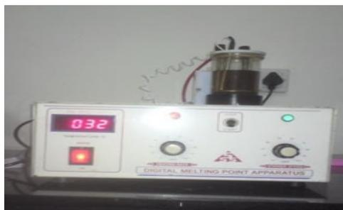
**Fig. 3:** Digital melting point apparatus
