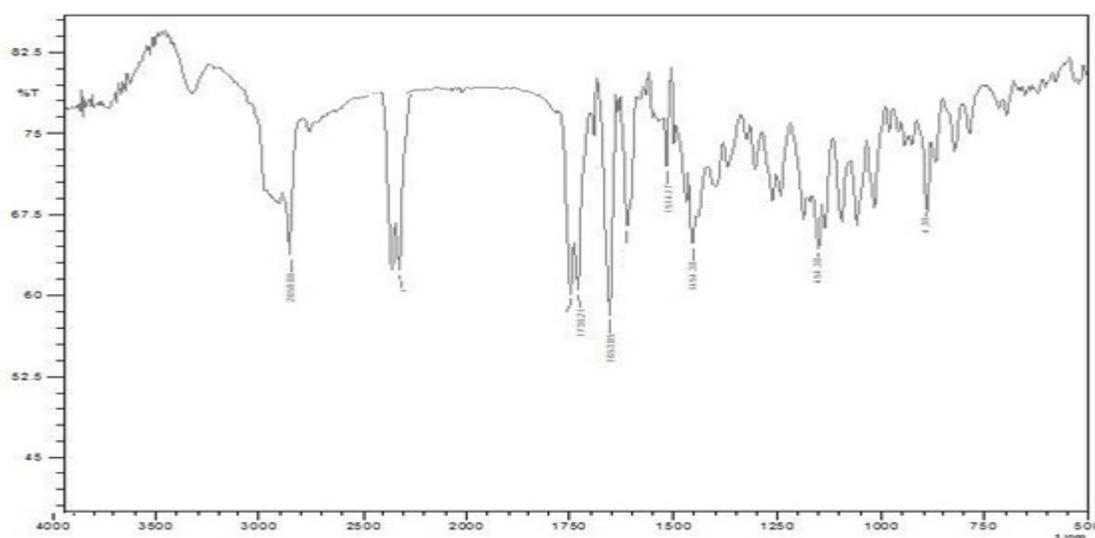
**Fig. 7:** FTIR spectra of Ipratropium bromide: Experimental
