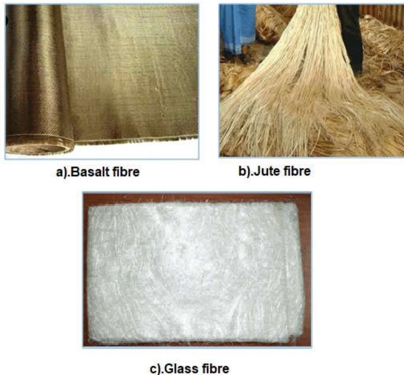
**Fig.1 Reinforcement Materials**
