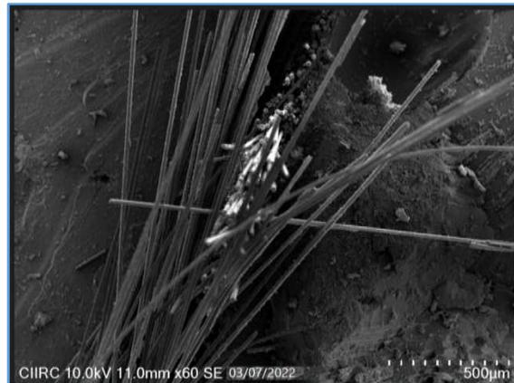
**Fig.6 SEM of Tensile Sample with Basalt and Glass Fibers before Failure**
