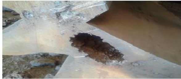
b. Sand sintering on gear component
