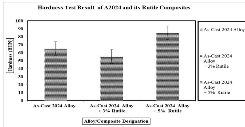
**Figure 3: Hardness values of Al2024 alloy and Its Composites**
