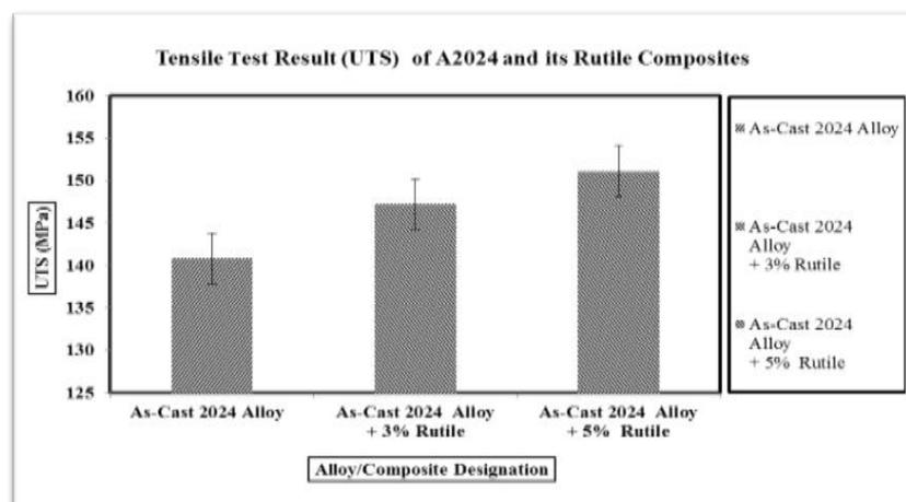
**Figure 4: UTS test results of Al2024 alloy and its Composites**
