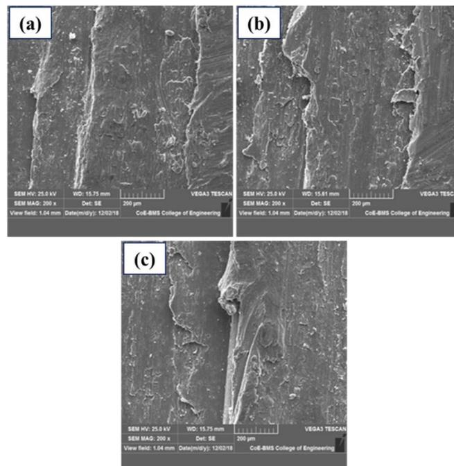
**Figure 9: Wear Surface Morphology of Al2024 grid alloy and its rutile composites. Where (a) Al2024 grid alloy at a load of 30N (b) Al2024 grid alloy+3% rutile at load of 30N (c) Al2024 grid alloy+ 5% rutile at a load of 30N**
