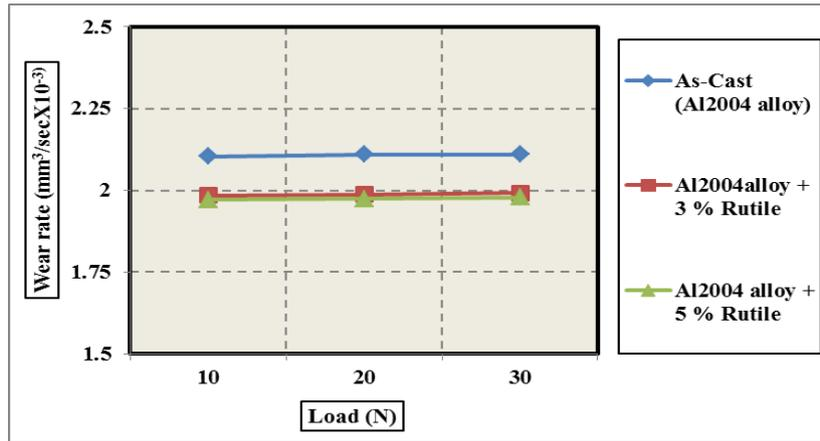
**Figure 8: Wear Rate vs Load of Al2024 grid alloy and rutile composites**
