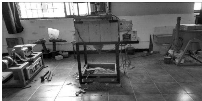
**Figure 1: Stir casting set-up assembly**
