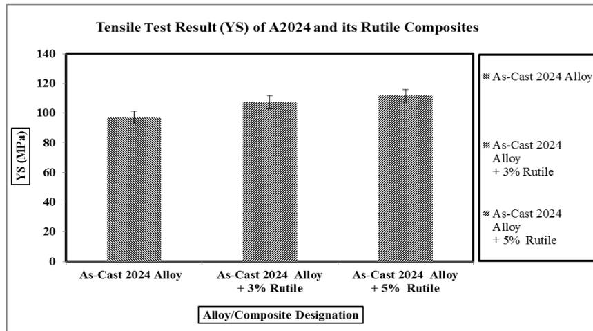
**Figure 5: YS test results of Al2024 alloy and its Composites**
