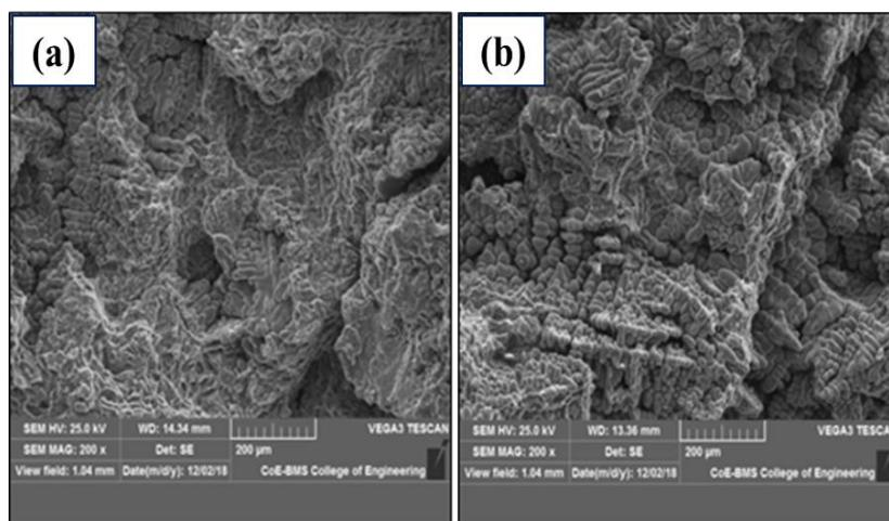
**Figure 7: Fractography of A2024 and its Rutile composites where (a): As-cast 2024 alloy (b) As-cast 2024 +5% Rutile**
