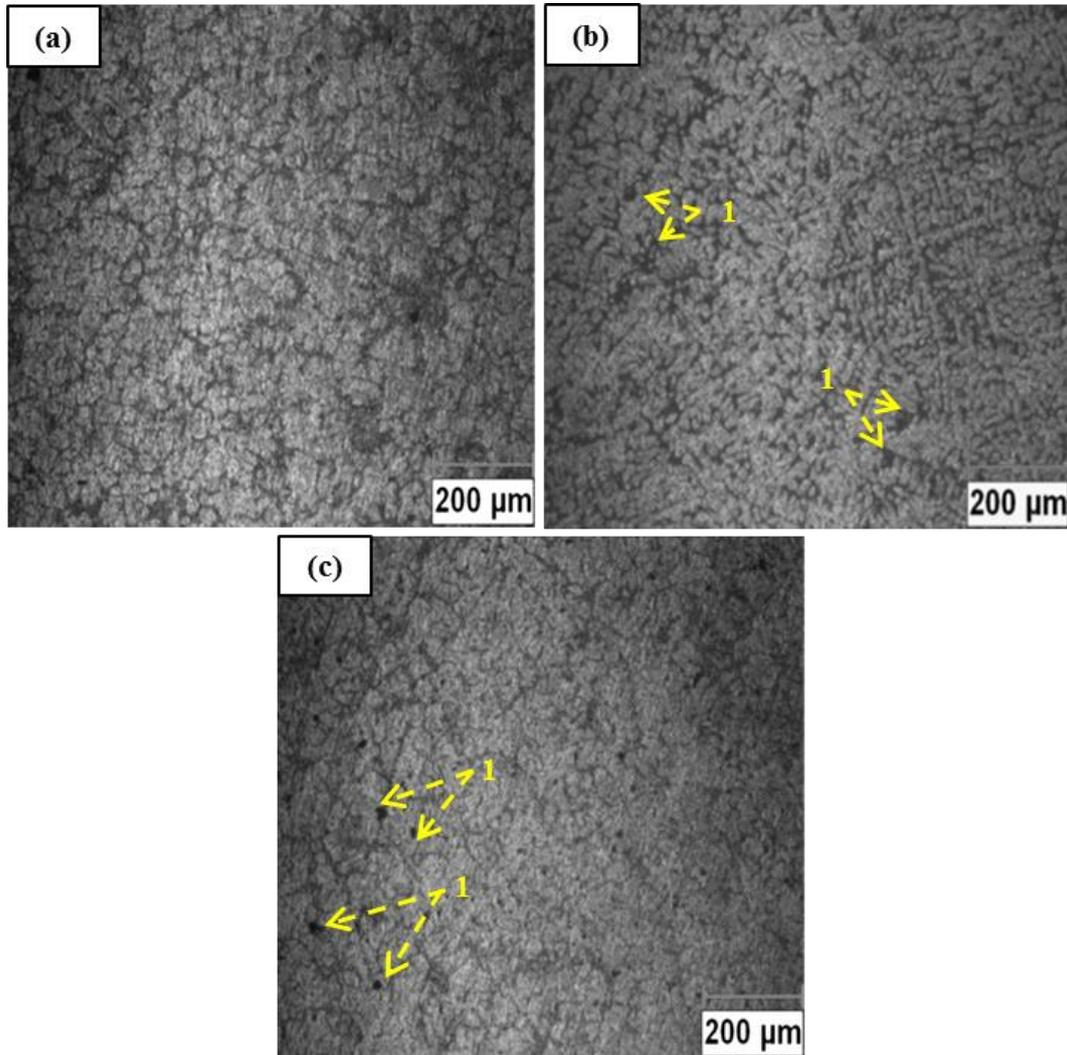
**Figure 2: Optical Micrographs of A2024 and its Rutile composites where (a): As-cast 2024 alloy, (b) As-cast 2024 +3% Rutile, (c) As-cast 2024 +5% Rutile**
