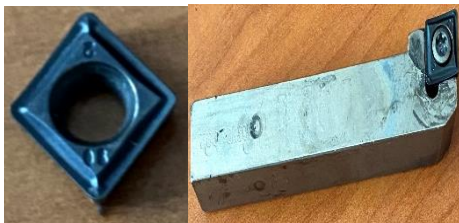
Fig. 2.1 Carbide Tool Insert and Tool Holder
