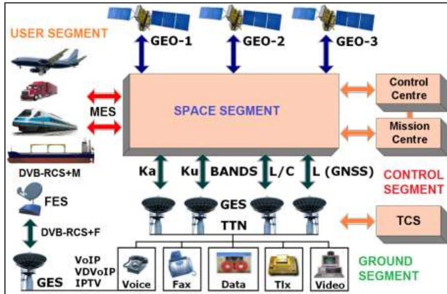
Fig. 4. Space, Ground and User Segments for Fixed and Mobile DVB-RCS System
