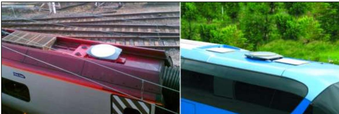
**Fig. 10.** The Phased Antenna Array Installed on the Roof of the Train and Bus
