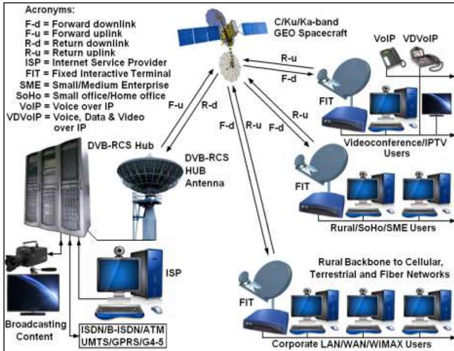
Fig. 3. DVB-RCS+F Backbone for Fixed Applications
