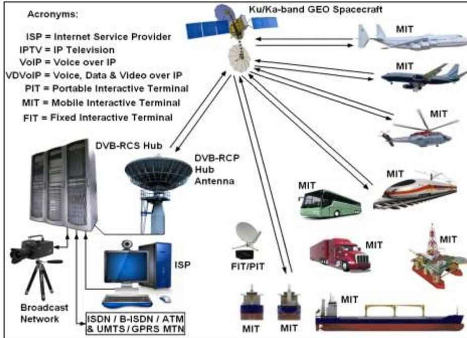
Fig. 5. DVB-RCS+M Backbone for Mobile Applications
