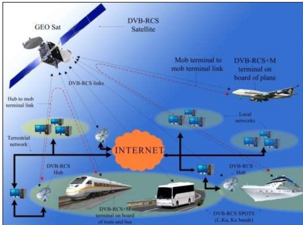
Fig. 6. Interactive Internet via DVB-RCS+M Backbone for Mobile Applications
