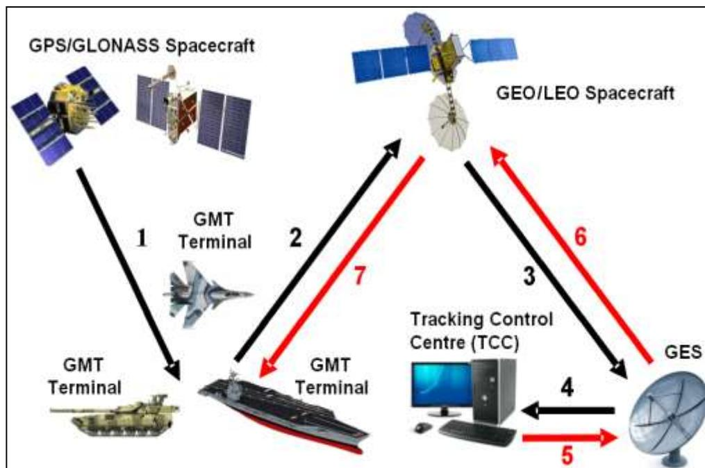
Fig. 4. Configuration of GMST via GNSS and GEO/Non-GEO Satellites
