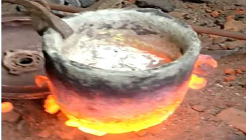
Figure4: Heating of Al- Al<sub>2</sub>O<sub>3</sub>/MgMMCs using Stir Casting
