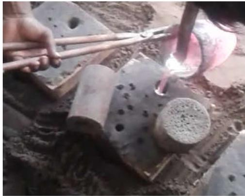
Figure 5: Pouring of molten metal in the mould
