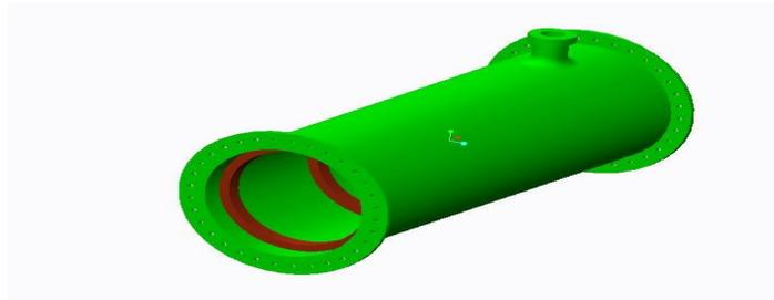
Fig3: TotalAssemblyBodyCoverandSurgePlates Assembly
