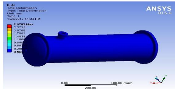
Fig.8 Deformation of the Cryogenic vessel Structural steel with Aluminum position
