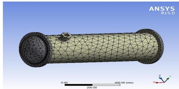
Fig. 7 Meshed model of the Cryogenic vessel Structural steel with Aluminum position
