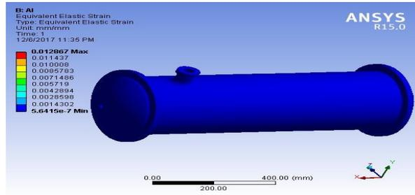
Fig.10 Equivalent Strain for the Cryogenic vessel Structural steel with Aluminum position
