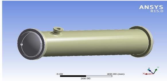
Fig 6. Geometry of the Cryogenic vessel Structural steel with Aluminum position
