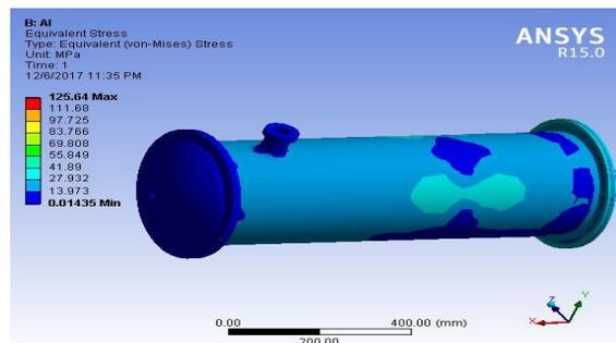
Fig.9 Equivalent Stress for the Cryogenic vessel Structural steel with Aluminum position
