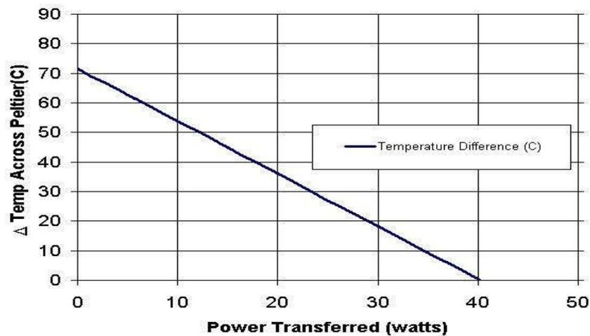
**Fig.3:** Power Vs Temp of Peltier plates
