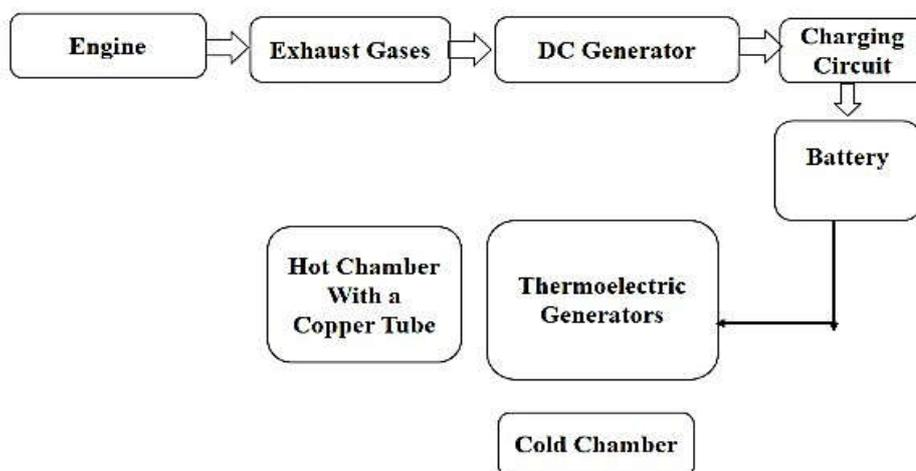
**Fig.1:** Block diagram of Waste Heat Recovery System
