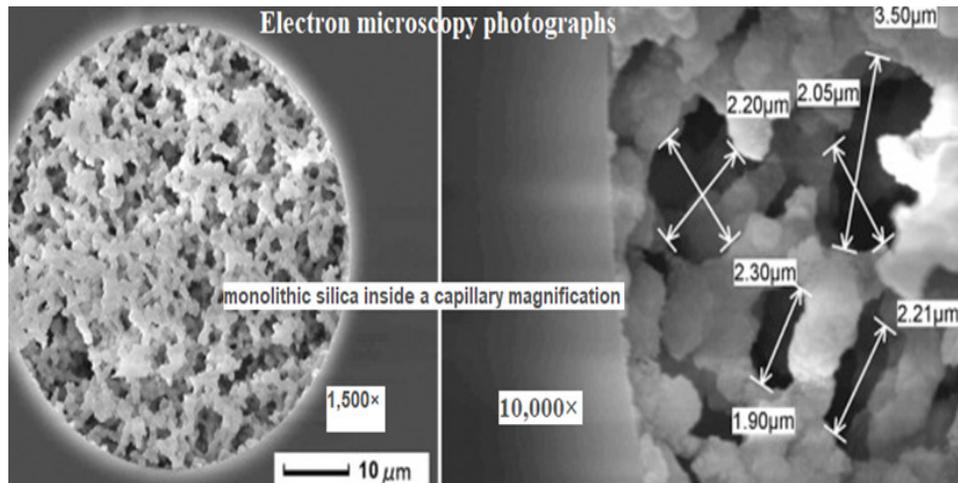
Fig. 1. Electron microscopy photographs of monolithic silica inside a capillary
