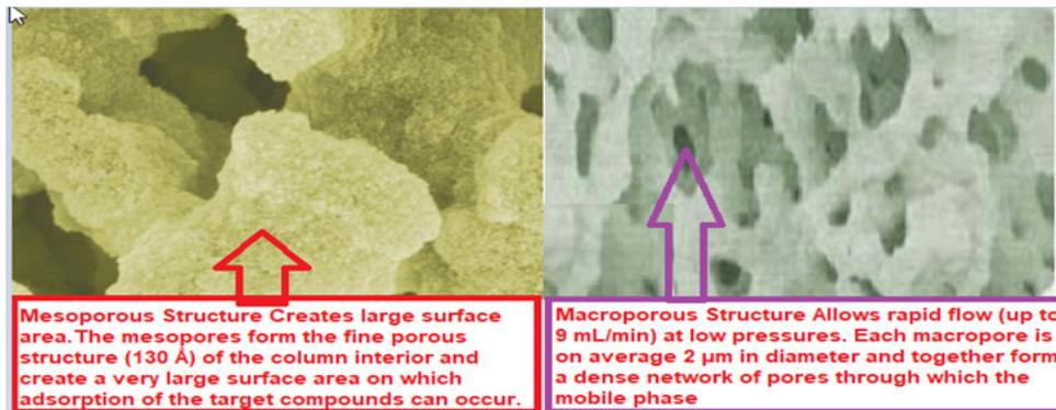
Fig. 2. Mesoporous and Macroporous revolutionary bimodal pore structures in monolithic HPLC column.
