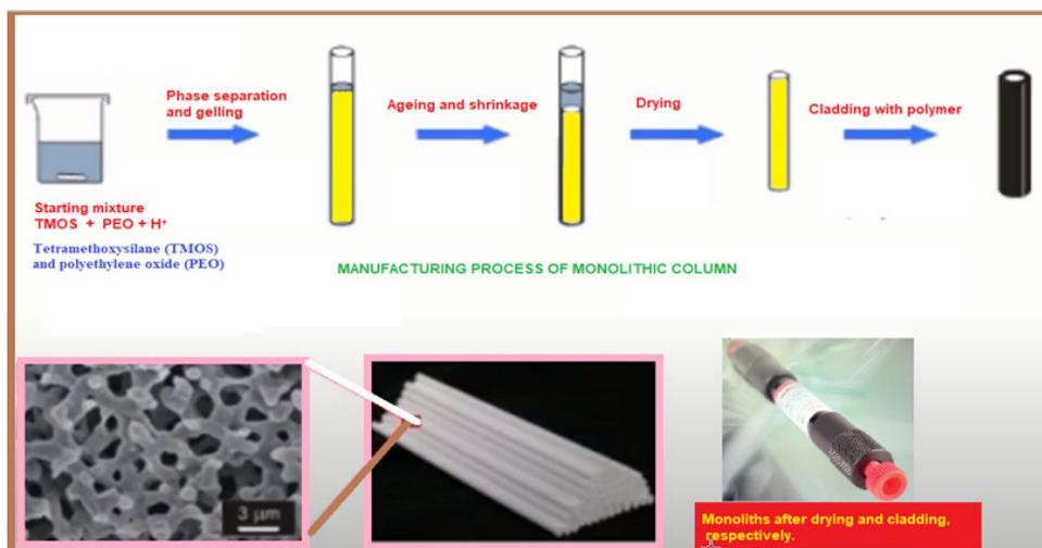
Fig. 4. The manufacturing process of the monolithic column.
