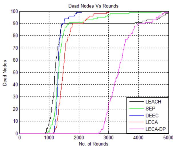
**Fig.12. Life span of Nodes in 2-level Heterogeneous Network (m:0.1,a:2)**
