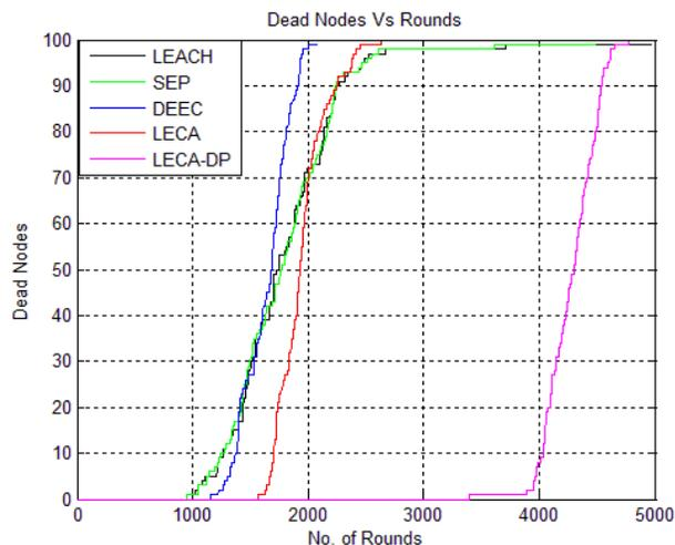
**Fig.11. Life span of Nodes in Multi-level Heterogeneous Network**
