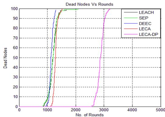
**Fig.10. Life span of Nodes in Homogeneous Network**
