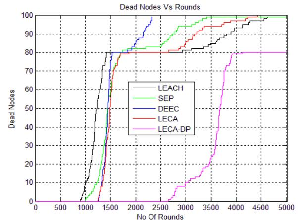
**Fig.13. Life span of Nodes in 2-level Heterogeneous Network (m:0.2,a:2)**
