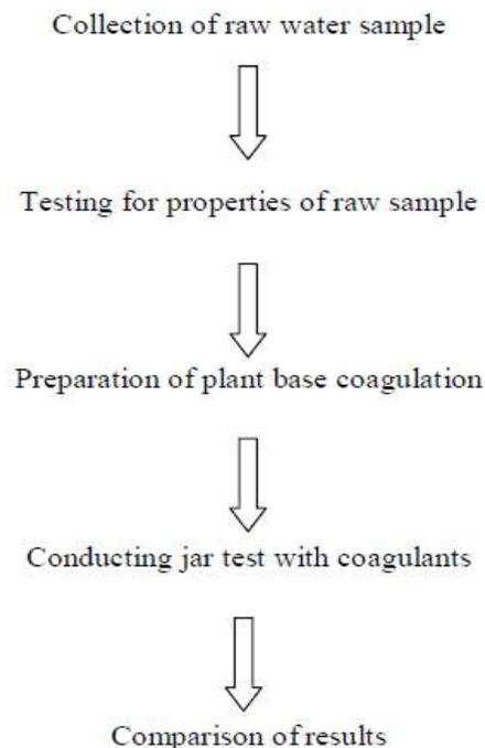
Water sample is collected from a lake located in Naknampur. The following tests were conducted on raw water sample to know its properties: pH, Turbidity, Conductivity, Alkalinity, Hardness, and Jar test. Tamarind seeds, Neem leaves, Chick peas, Drumstick seed powder were the materials used in the experiment. The process of preparation of coagulant is explained below.
