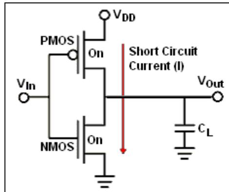
Figure 4. Dynamic Internal Power Loss
