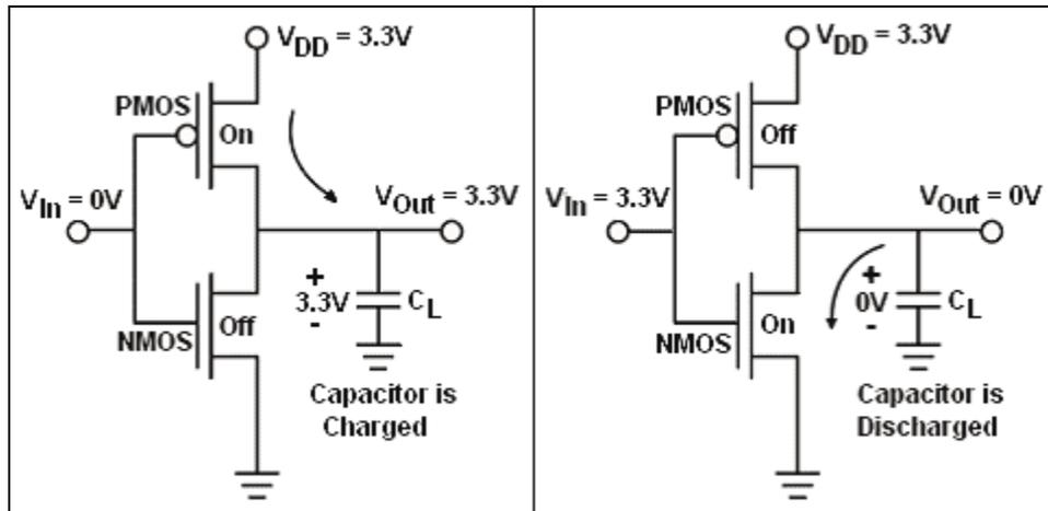
Figure 3. Dynamic Switching Power Losses
