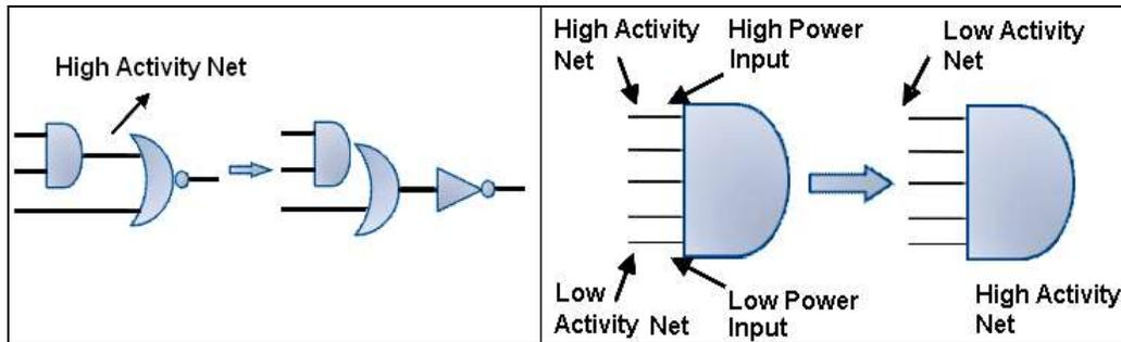
Figure 8. Gate Level Optimization Technique
