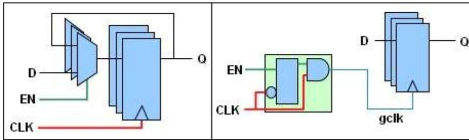
Figure 6. Two Types of Clock Gating Technique
