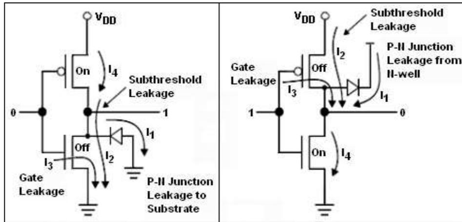
Figure 5. Static Leakage Power Loss
