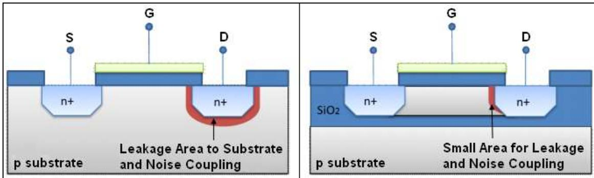
Figure 10. SOI CMOS Devices Technique
