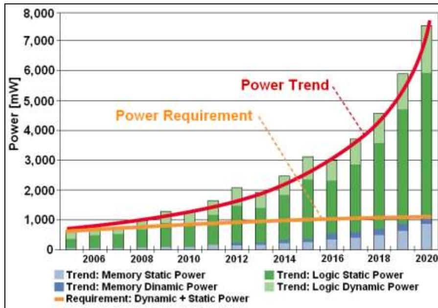
Figure 1. Bulk-CMOS Trend in Smart Home Applications
