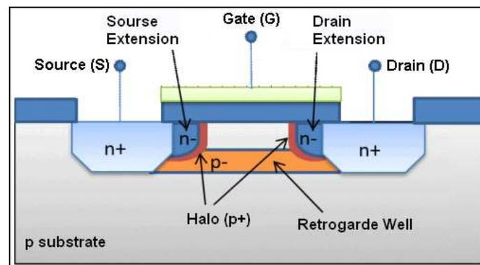
Figure 9. Retrograde and Halo Doping – Bulk CMOS Technique
