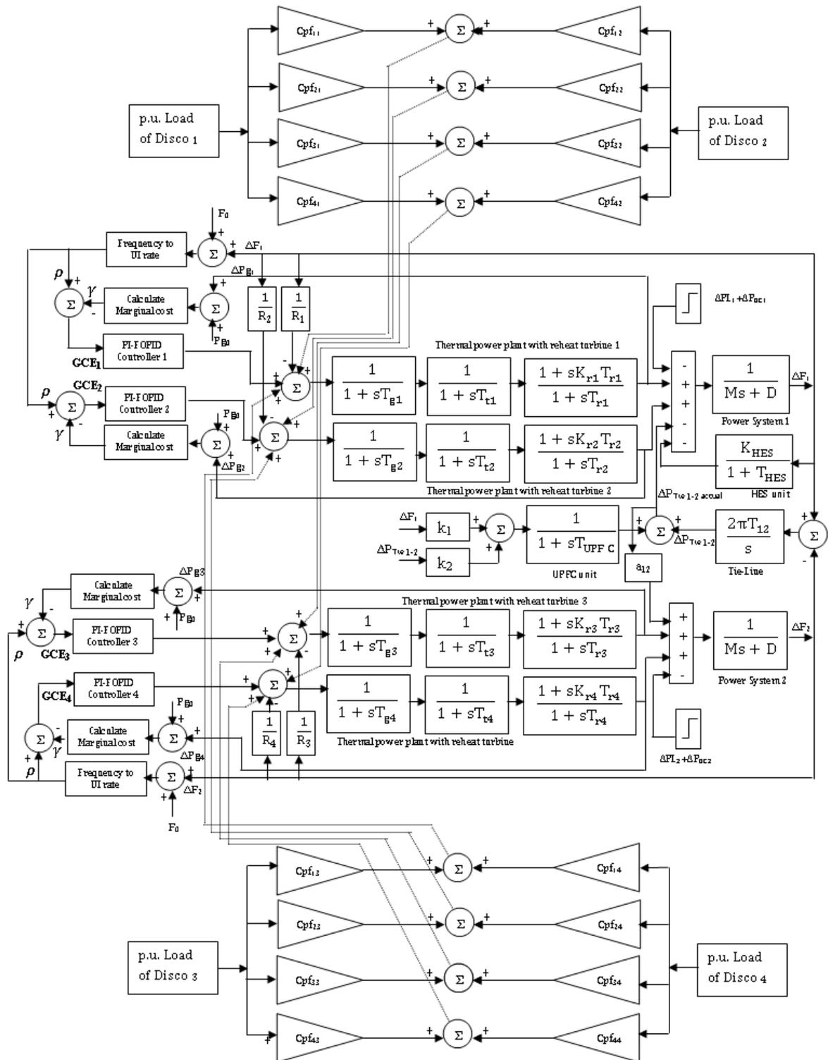
**Fig. 6. Transfer function model of Price signal based Automatic Generation Control loop for a two area thermal-thermal deregulated power system with HES and UPFC units**
