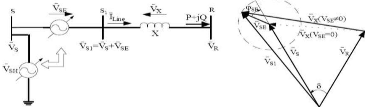
**Fig. 5 Application of UPFC unit in the tie-line**
