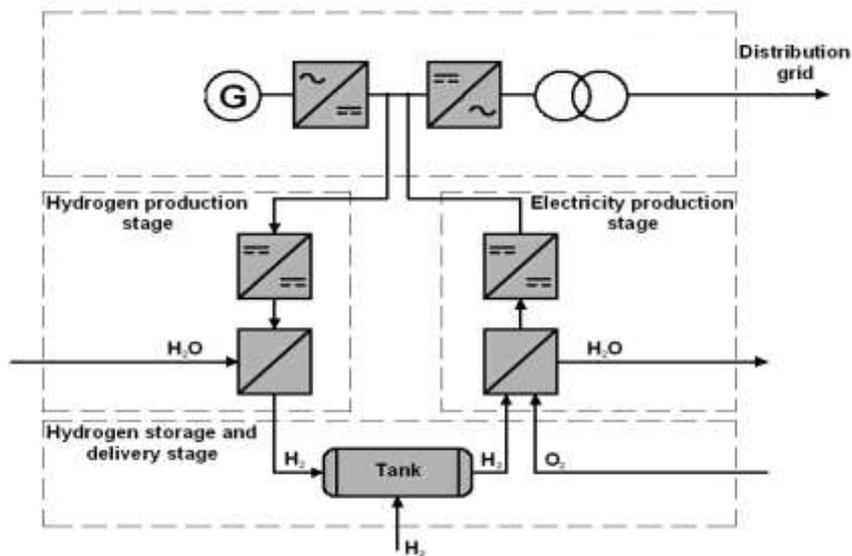
**Fig. 3 Block diagram of the Hydrogen Energy Storage unit**
