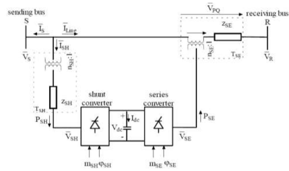
**Fig. 4 Unified Power Flow Controller configuration**
