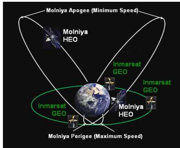
**Figure 5.** Hybrid GEO and HEO Satellite Constellations –
