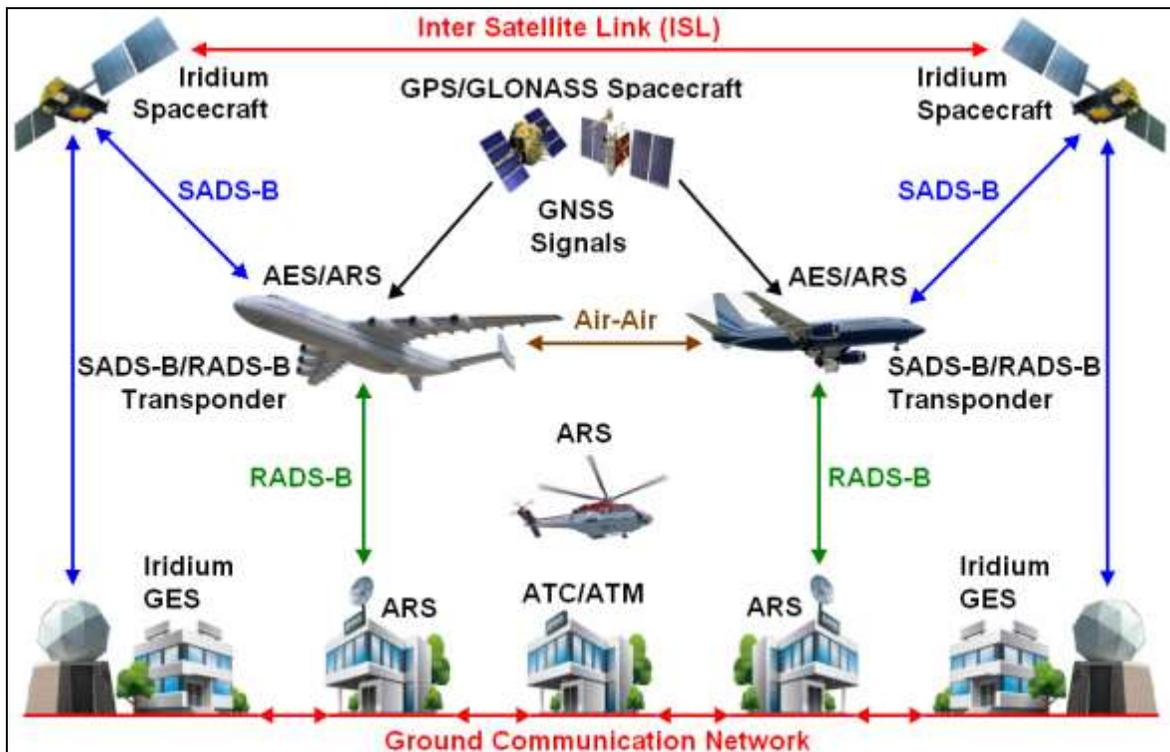
Figure 8. Aeronautical Iridium Surveillance Network – Courtesy of Manual: by Ilcev
