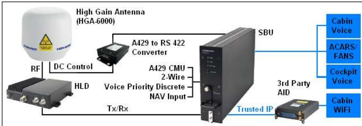
**Figure 2.** Airborne Inmarsat SwiftBroadband-Safety (SB-S) System – Courtesy of Manual: by Cobham
