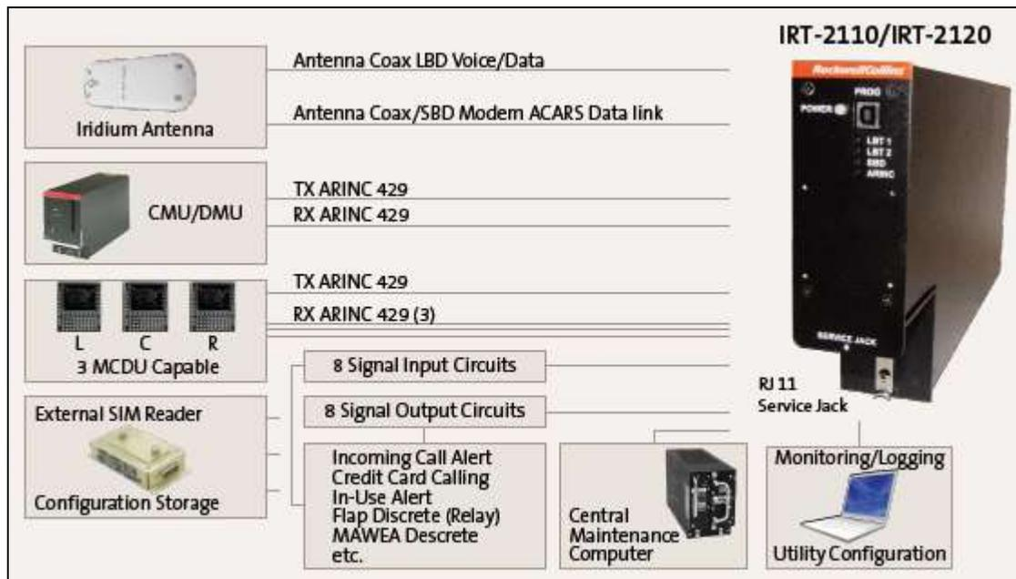
**Figure 9.** Aeronautical Iridium Communication System – Courtesy of Manual: by Rockwell Collins
