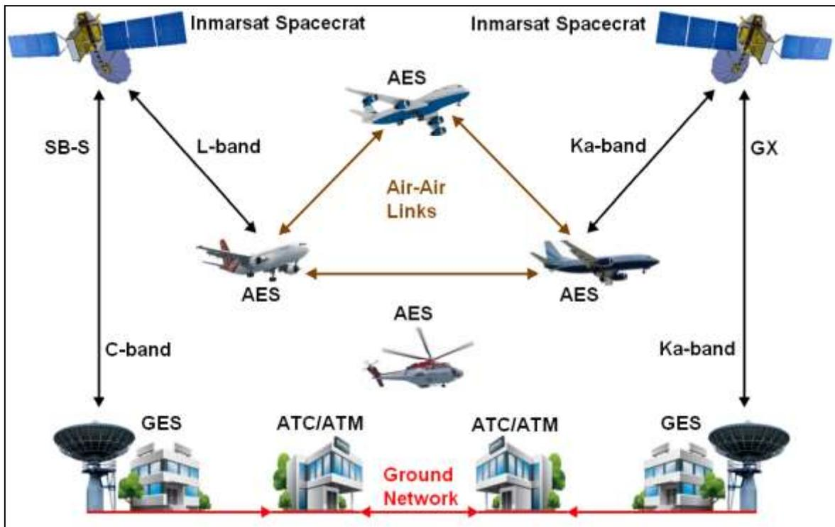
**Figure 1.** Aeronautical Inmarsat Communication Network – Courtesy of Manual: by Ilcev
