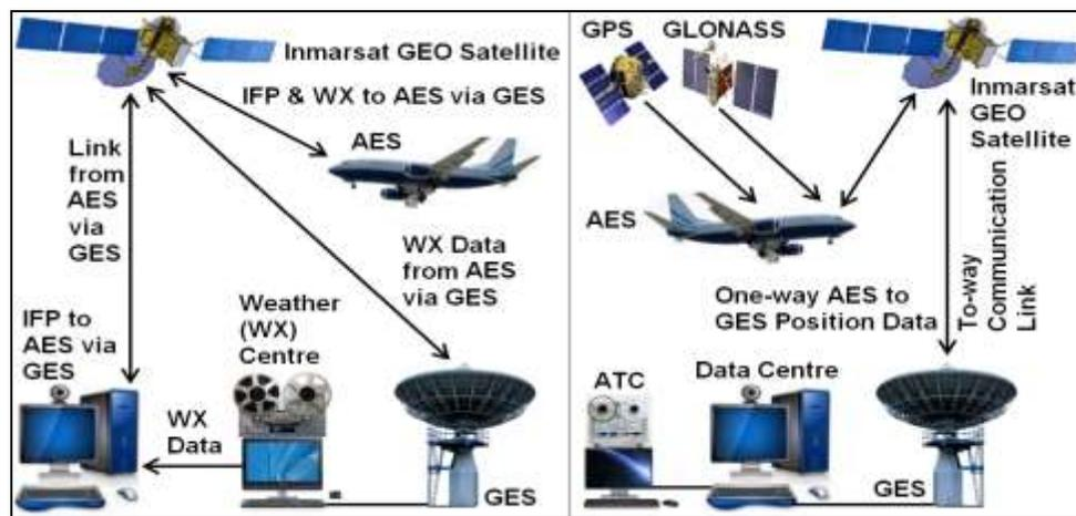
**Figure 4.** Aeronautical Weather and S-ADS Solutions via Inmarsat –
