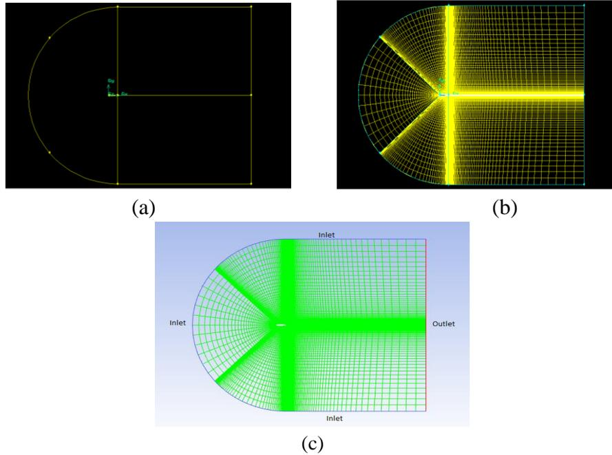
Figure 2: a) Geometry and dimensions of Computational domain in Gambit 2.4.6
