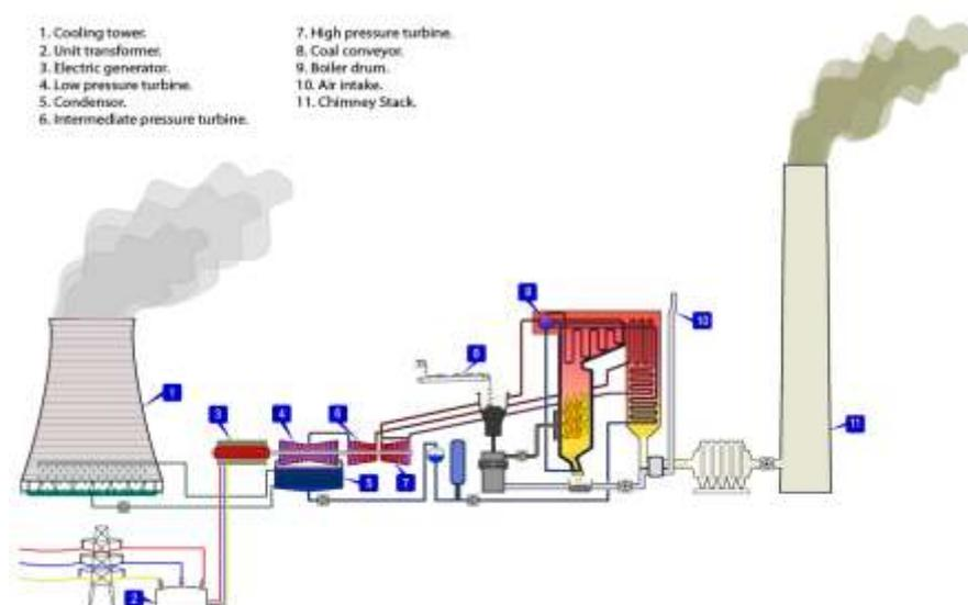
Fig 1: Thermal Power Plant Layout
