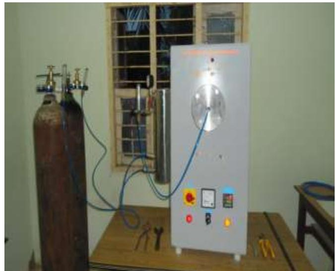
Fig 5: Furnace with CO<sub>2</sub> and O<sub>2</sub> cylinder arrangement
