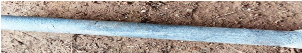
Figure 2: carbon steel recycled cast rod
