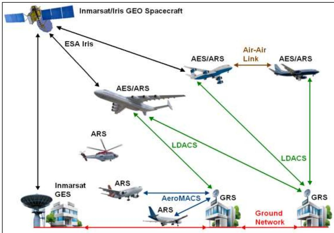
Figure 6. Integration of Satellite, LDACS and AeroMACS Networks – Courtesy of Manual: by Ilcev
