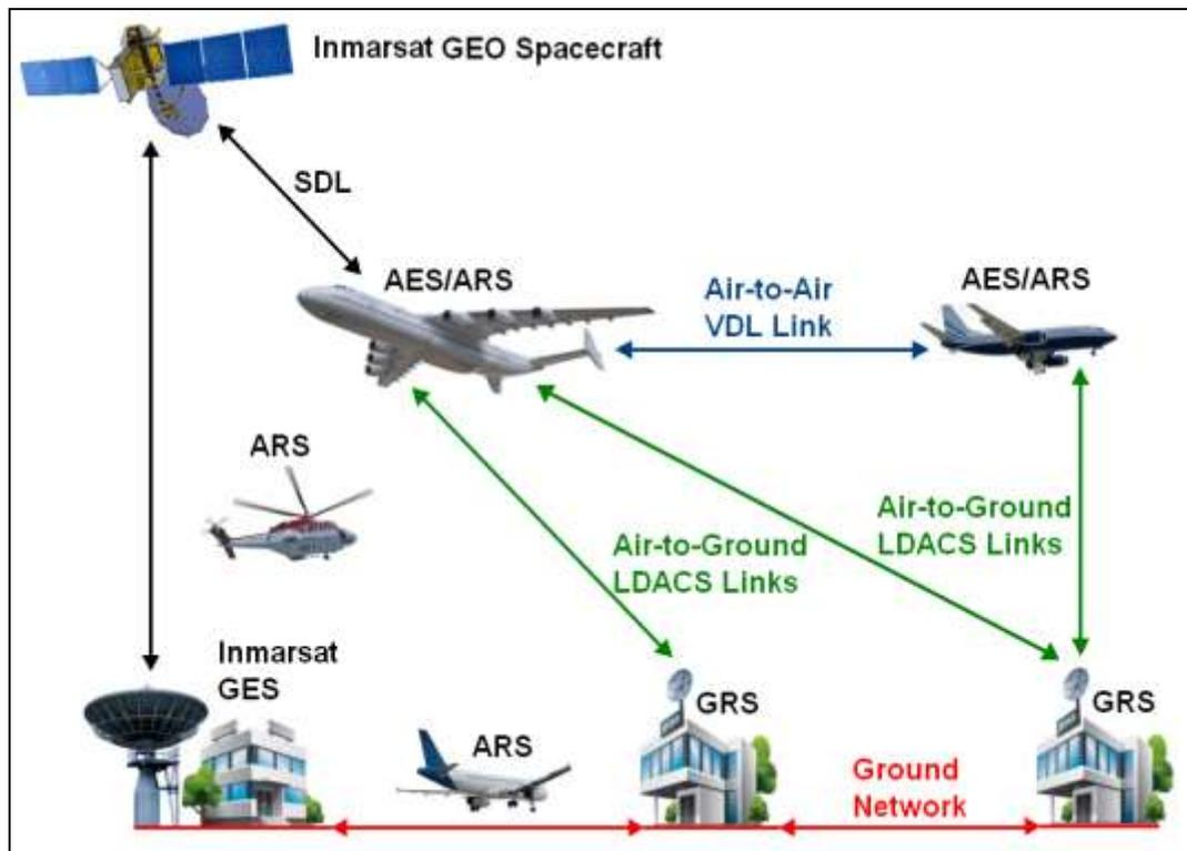
**Figure 7.** Integration of Satellite, LDACS and VDL Networks – Courtesy of Manual: by Ilcev
