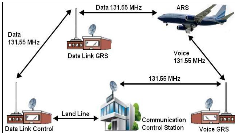
Figure 2. Radio VHF ACARS Network – Courtesy of Manual: by Ilcev
