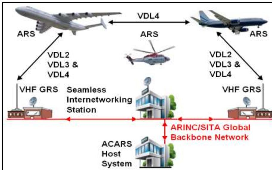
Figure 3. Radio VDL Communication Network – Courtesy of Manual: by Ilcev
