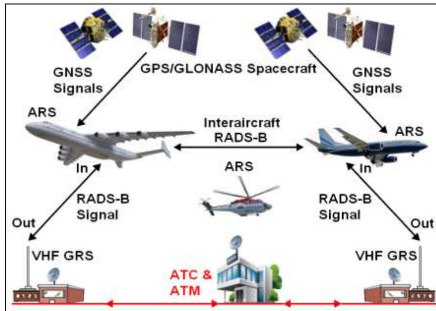
Figure 4. Radio ADS-B CNS Network – Courtesy of Manual: by Ilcev
