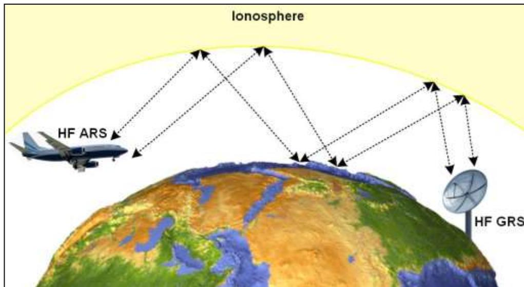
**Figure 5.** Radio Communications via HF-band – Courtesy of Manual: by Ilcev
