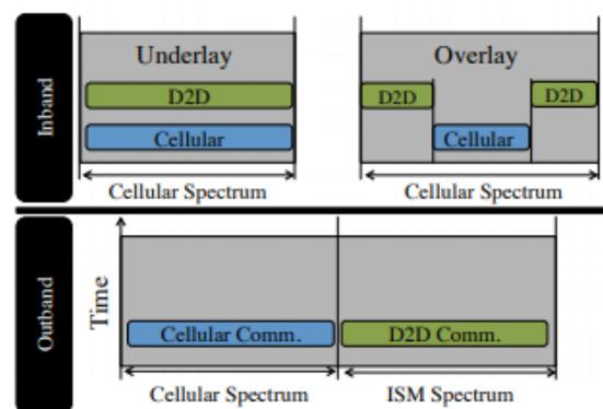
**FIGURE.2: Schematic representation of overlay inband, underlay inband, and outband D2D**
