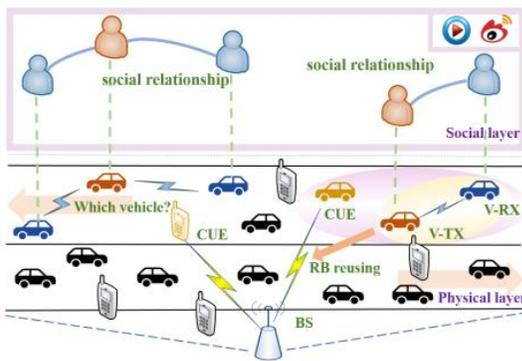
**FIGURE.1: The physical layer and social layer models of D2DV2V based IoV networks**
