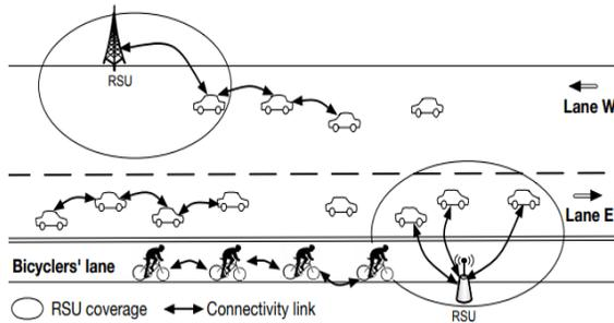
**FIGURE.2: Schematic of a vehicular ad hoc network**
