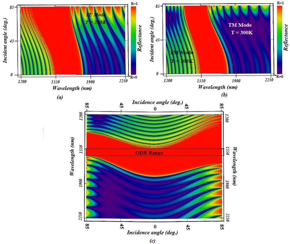
Fig. 2.ODR spectrum of 1D photonic crystals (ZnS/GaAs) at different angle of incidence at  $T=300K$ .
