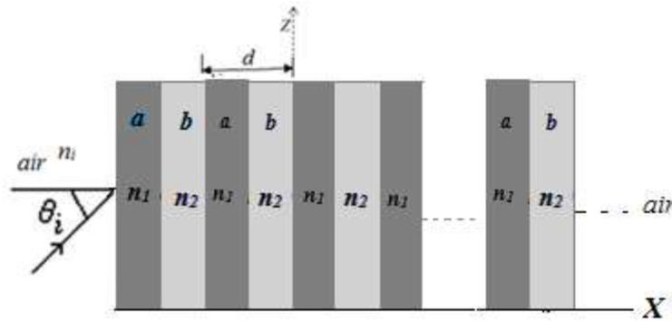
Fig.1. Structure of one-dimensional photonic crystals.
