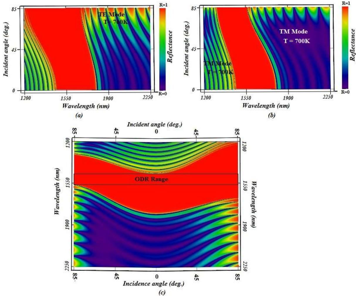
Fig. 3.ODR spectrum of 1D photonic crystals (ZnS/GaAs) at different angle of incidence at  $T=700\text{K}$ .
