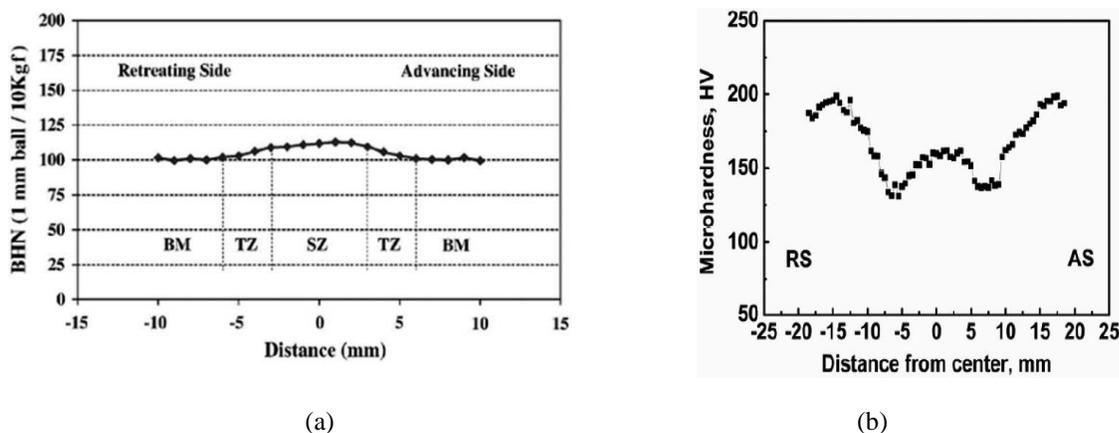
Figure 12 Micro hardness profile reinforced with SiC particles for (a) A356 and (b) AA2009 [34]
