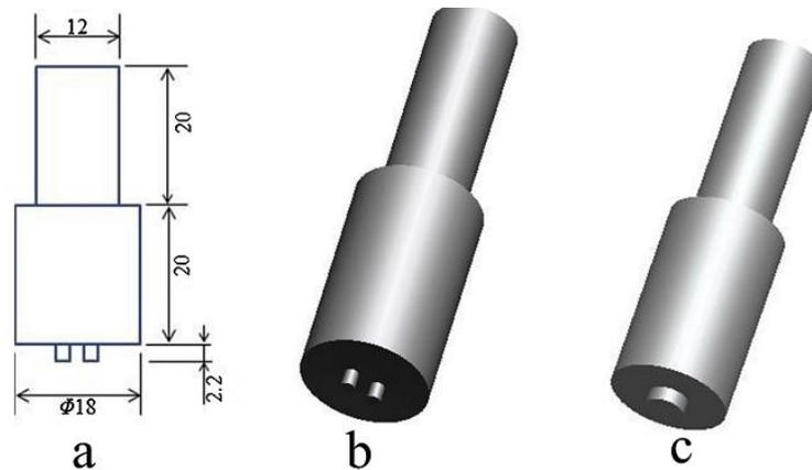
Fig. 6 Geometry and dimension of applied tools: (a –b) dual-pin tool, (c) single-pin tool [9].
