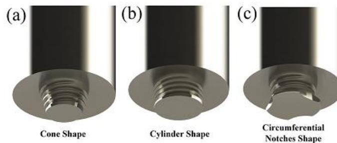
Fig. 5 Illustration of three designed probe geometries: (a) cone shape, (b) cylinder shape & (c) circumferential notches shape
