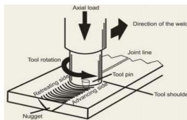
Fig. 1 Friction Stir Welding [3]
