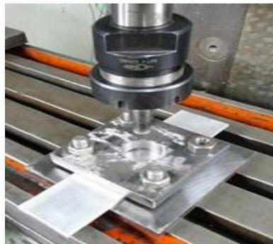
Fig. 13: Friction Stir Spot welding system and clamping device [16]
