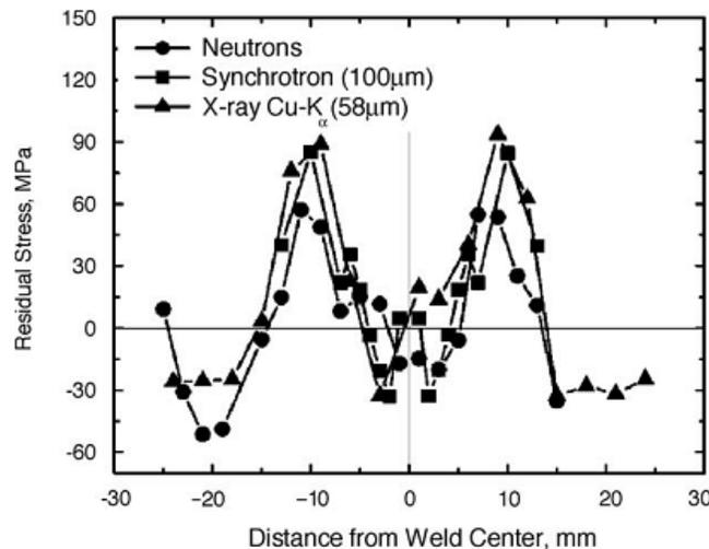
Fig. 11 Longitudinal residual stress distribution in FSW 6013Al-T4 welds determined by different measurement methods (tool rotation rate: 2500 rpm, traverse speed: 1000 mm/min tool shoulder diameter: 15 mm) [32]
