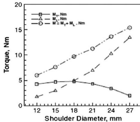
Fig. 4 Variation of Sliding, Sticking and Total Torque with Shoulder Diameter [29]
