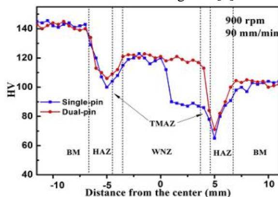
Fig. 9 Vicker's micro-hardness profiles of the cross-section of dissimilar joints produced by single-pin and dual-pin tool [9].
