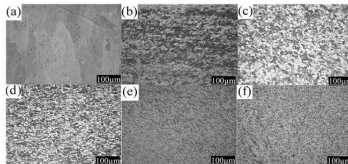
Fig. 7 Optical micrographs of AA2219 FS Welds of Nugget Zone (a) Base metal (b) Conical tool (c) Triangle tool (d) Square tool (e) Pentagon tool and (f) Hexagon tool [11].
