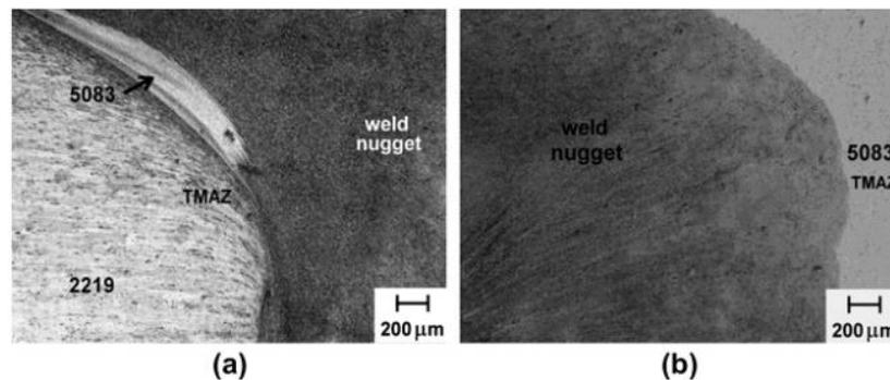
Fig. 10 TMAZ microstructures: (a) advancing, & (b) retreating side [5].
