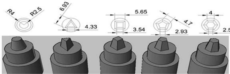
Fig. 2 Geometry of tool profiles [11]
