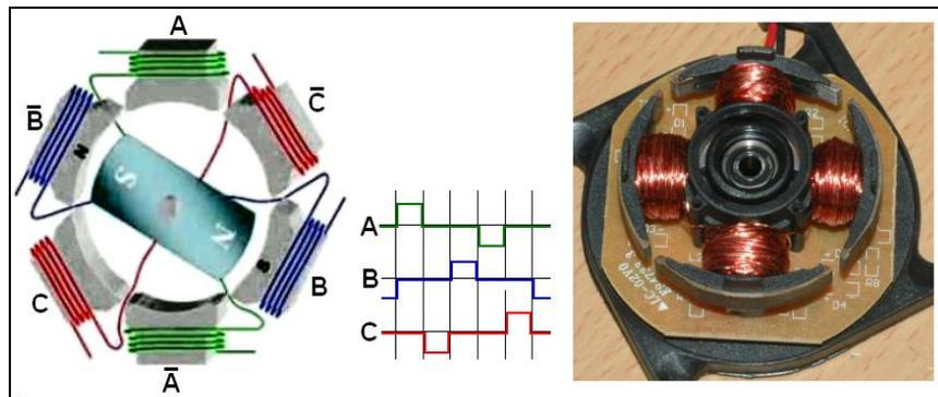
Figure 8. BLDC Motor and Permanent Magnet Rotor
