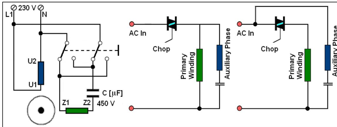
Figure 4. Single Phase Asynchronous Motor and Speed Regulation
