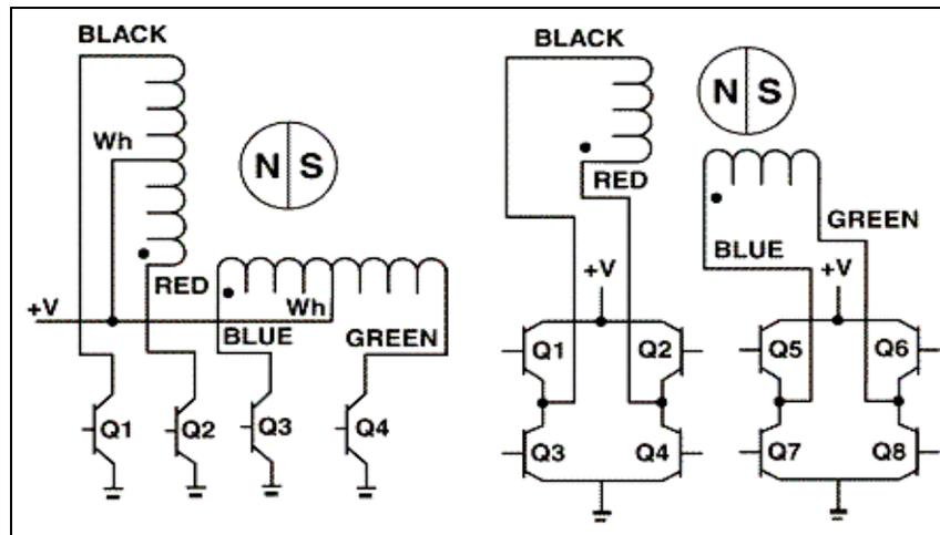
Figure 11. Unipolar and Bipolar Stepper Motors
