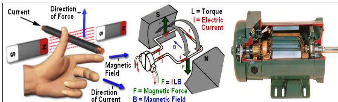
Figure 7. Fleming’s Left Hand Rule and DC Motor
