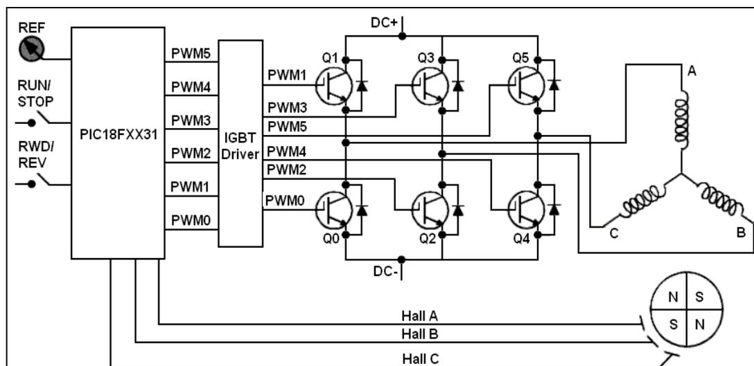
Figure 9. Block Diagram of BLDC Motor
