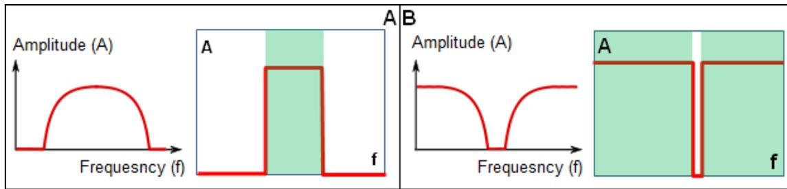
**Figure 4.** Amplitude Spectrum of Bandpass and Bandstop Filters
