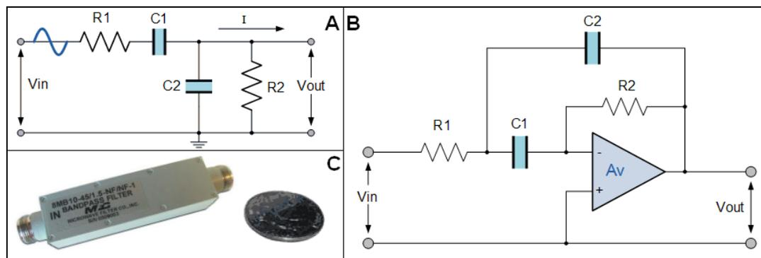
Figure 3. Circuits and Product of Passive and Active Bandpass
