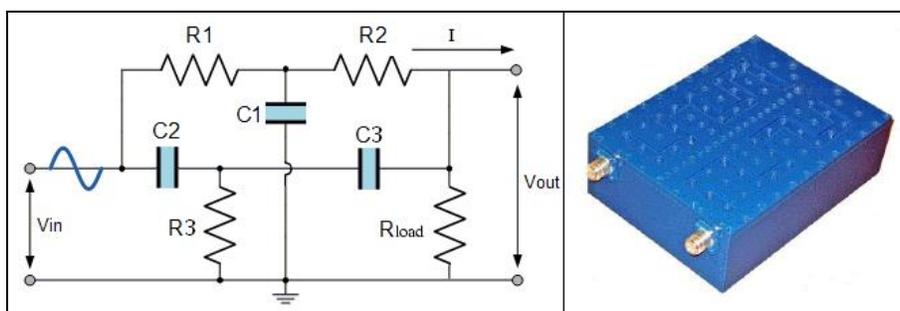
**Figure 5.** Circuits and Product of Bandstop Filter
