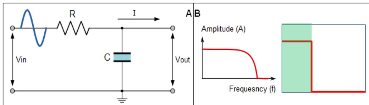
**Figure 8.** Circuits and Amplitude Spectrum of Lowpass Filters
