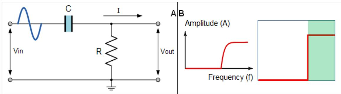
**Figure 6.** Circuits and Amplitude Spectrum of Highpass Filters
