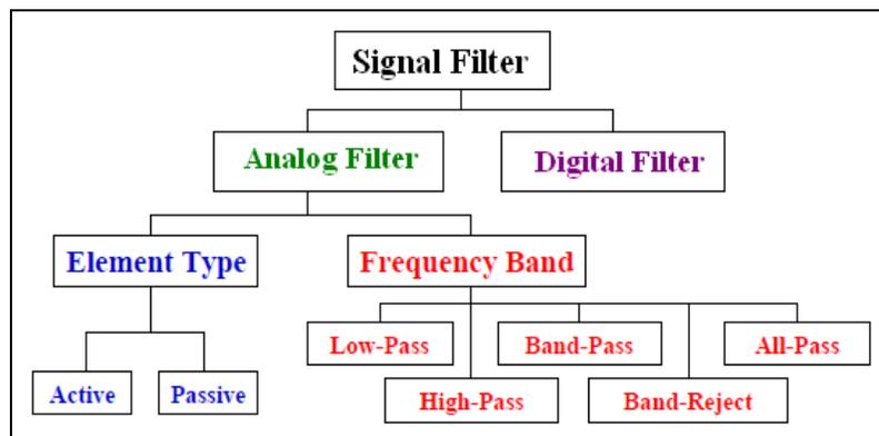
**Figure 1.** Classification of MW and RF Filters
