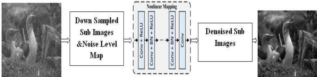
**Fig.1. The architecture of the proposed FFDNet for image denoising. The input image is reshaped to four sub-images, which are then input to the CNN together with a noise level map. The final output is reconstructed by the four denoised sub-images.**
