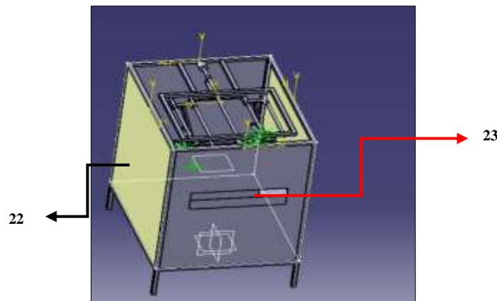
**Figure (d): Outer rectangular frame isolated with sheet metal covering**
