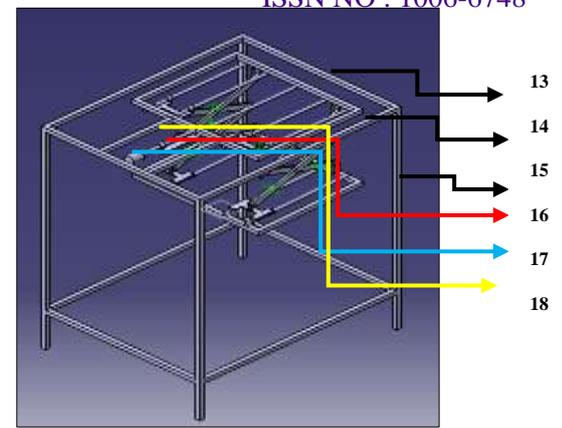
**Figure (c): Outer rectangular frame welded with whole scissor mechanism**
