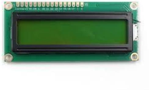
**Fig-3: 16X2 LCD Display**
