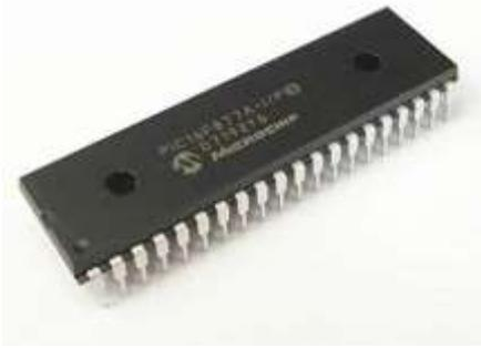
**Fig.4 PIC Microcontroller**
