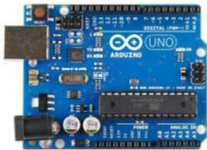
**Fig.5 .Arduino Uno Board**
